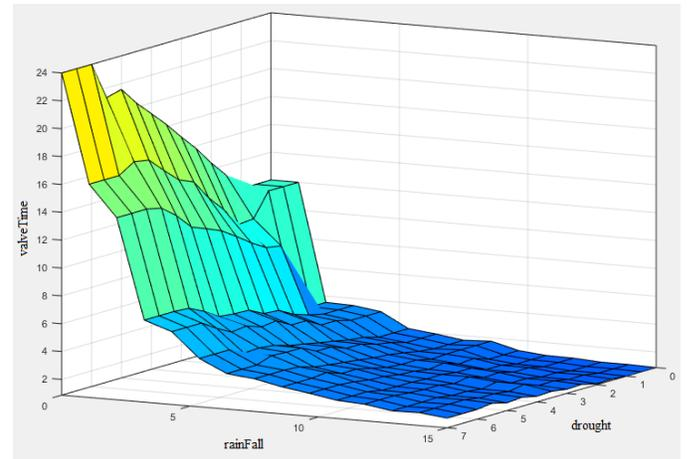
Fig.7. Control surface based on the rules
