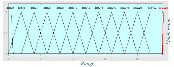
Fig.6. Output membership function valveTime
