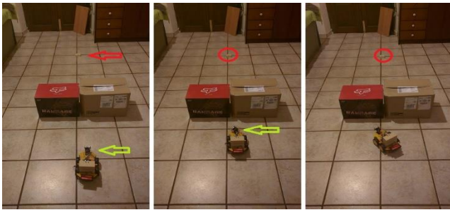
Figure 9 :1 st part of the algorithm-obstacle detection
